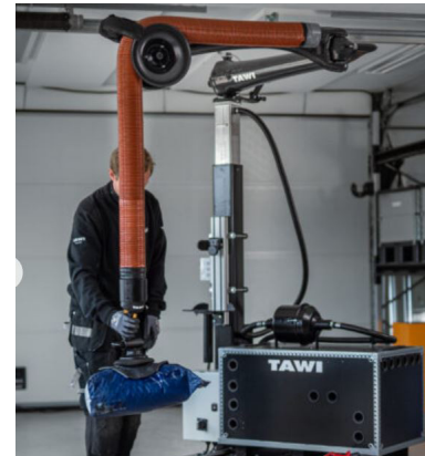
The Mobile High Frequency Lifter in use
